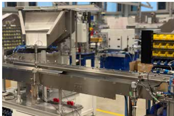
Typical application: SLL 804 Z-1600 as accumulation and feeding section in the pharmaceutical industry
