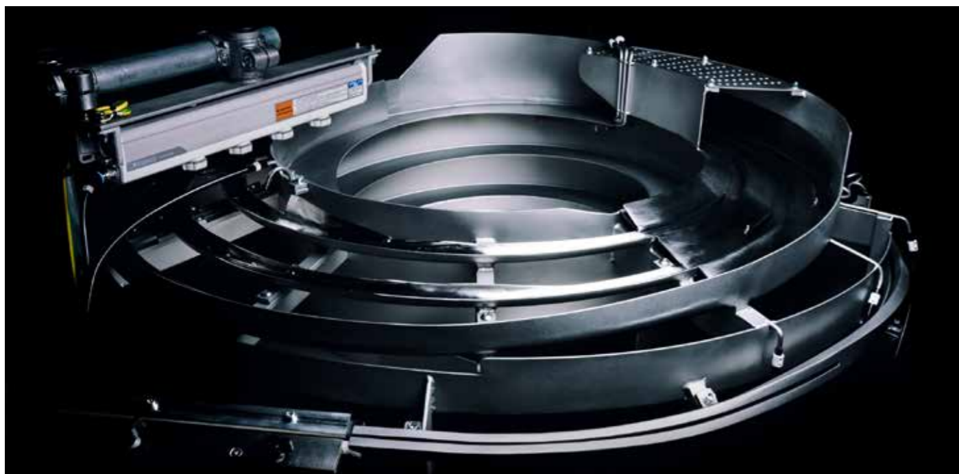
Typical application: SRHL 400-1 with ZSB-BA 400 for multi-lane feeding of plastic parts
