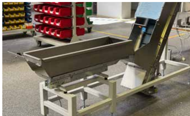
Typical application: BVL-25 SE for metered feeding of pins to an incline conveyor
