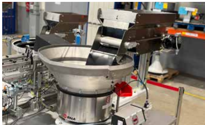
Typical application: Feeding system with BUW-25 for metered filling
