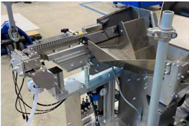
Typical application: SLA 400-400 with linear sorting device in combination with an STS nano step feeder
