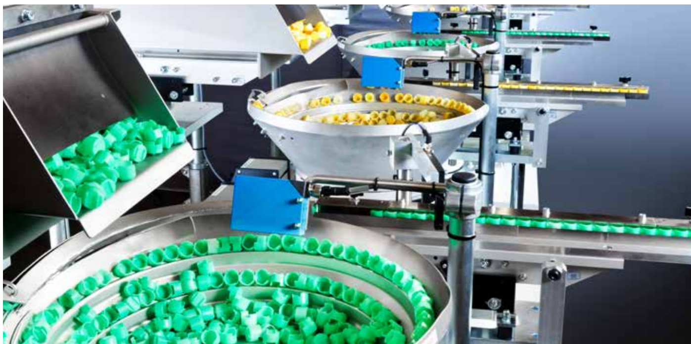
Typical application: SRC-N 250-2 with KSB-N 250 and closed spiral track for feeding of caps
