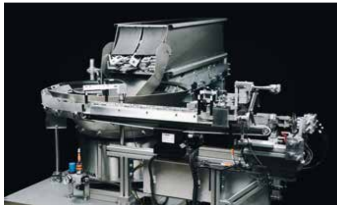
Typical application: Feeding system with BVL-5 for metered filling of the feeder bowl
