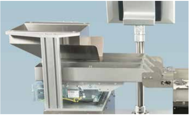
Typical application: Two 2 BVL-3M with static hopper for metered filling of a vibratory platform
