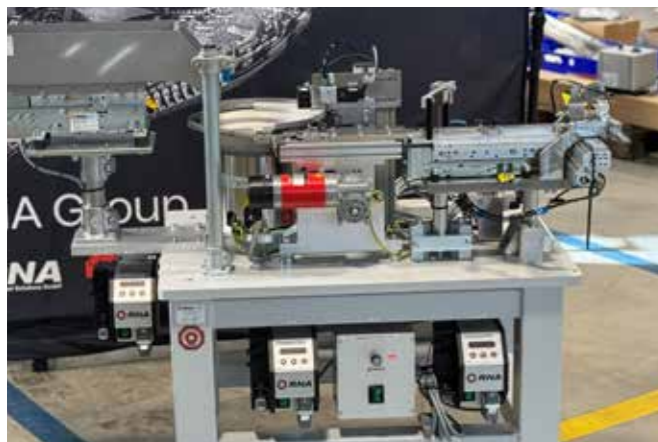
Typical application: SLL 175-250 as accumulation section for feeding to an escapement
