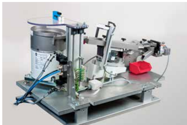
Typical application: Feeding system with SLS 250 for pins
