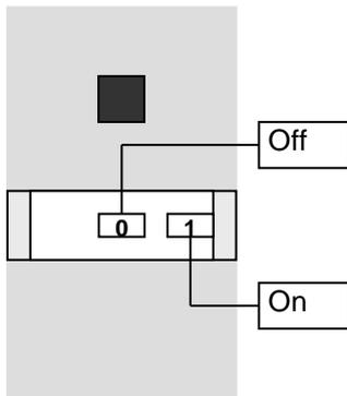
Fig. 6: Motor protection breaker
