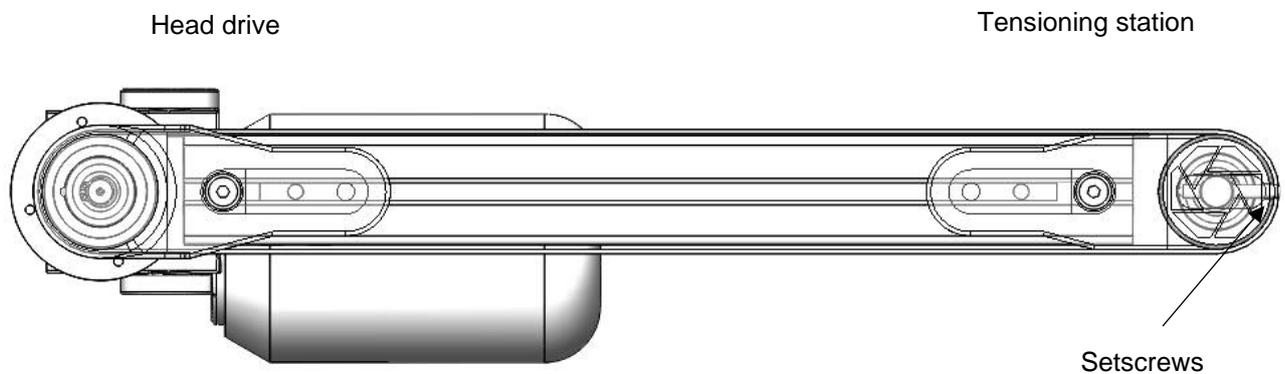
Fig. 9: Replacing a belt with head drive station
