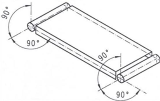
Fig. 5: Roller alignment
