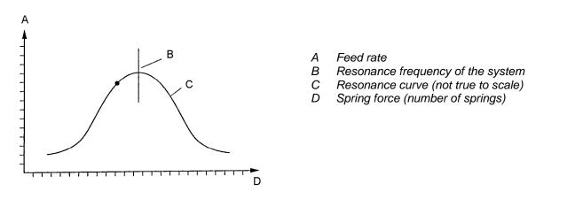
**Notice** The resonance frequency of the linear feeder must not be equal to the mains frequency.
