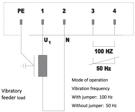
With jumper: The jumper must be inserted between connections 3 + 4.
