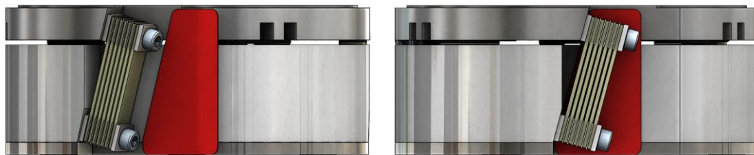
Installation of spring pack
